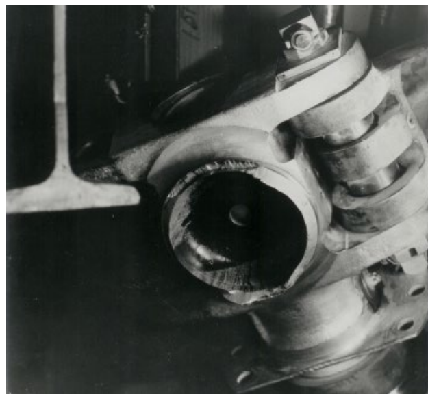
Figure 4 View of Fatigue Failure at MLG Strut Radius
