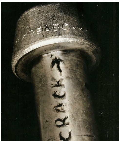
Figure 3 View of Cracked Tension Bolt
